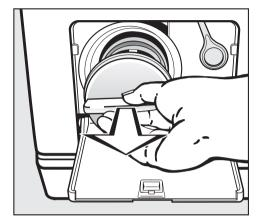
Remove any foreign objects (e.g. buttons, coins, etc.) and fluff from the filter housing. Turn the impeller by hand to check that it rotates freely. Any foreign object causing an obstruction should be removed.
